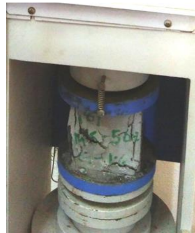
Fig. Cube after failure in compressive testing machine
