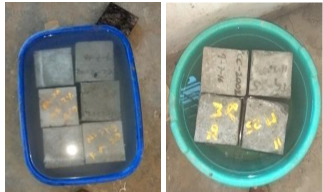
Fig. Cubes cured in Acid and Base
